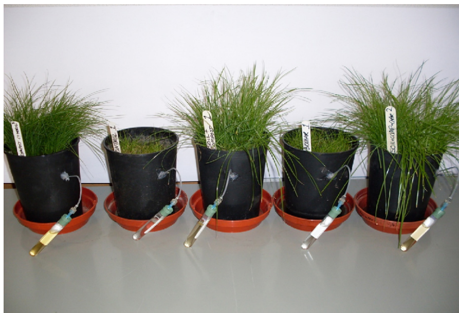
Fig. 1. Experimental set-up showing rhizon samplers collecting pore water and differences in ryegrass growth between soil and treatments 7 weeks after germination, from left to right; green waste compost reference, untreated soil, soil plus green waste compost, soil plus biochar, soil plus green waste compost and biochar. Note that only one of the triplicates of each treatment is shown.
